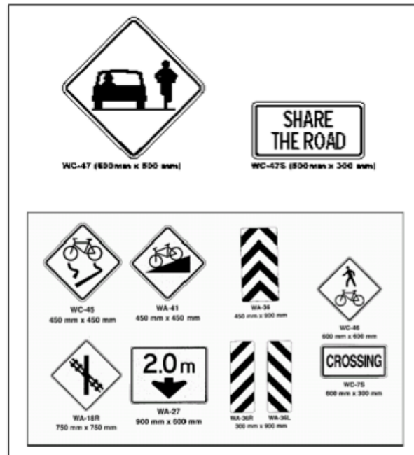
Examples of Warning Signs (Source: Bikeway Traffic Control Guidelines for Canada, Transportation Association of Canada, 1998)
